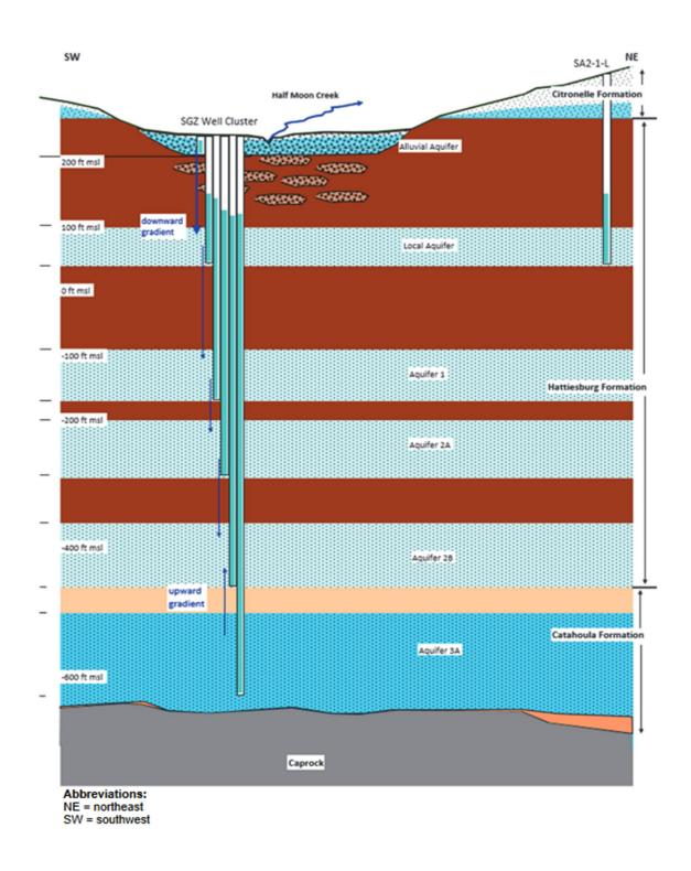
Figure 23. Conceptual Model of the SGZ Well Cluster
