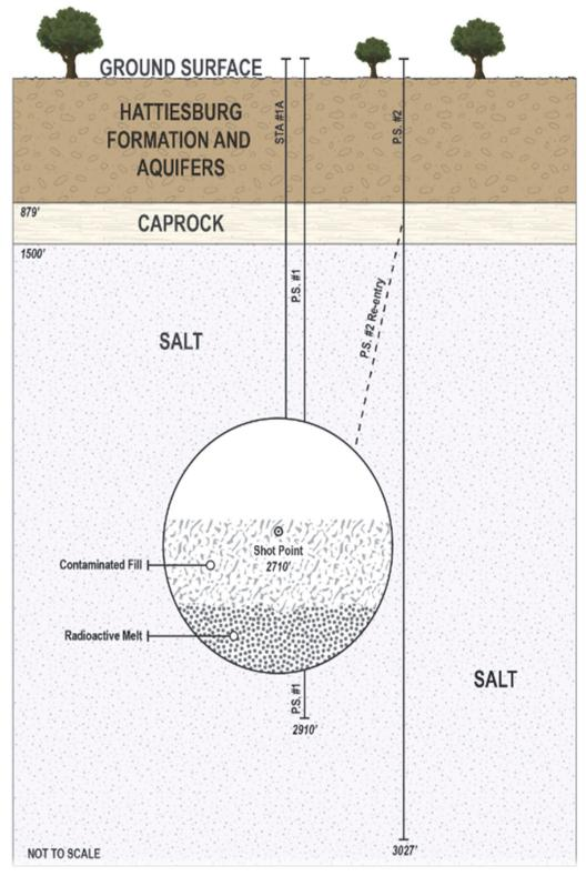
Figure 24. Cross-sectional Depiction of the shot Cavity After Surface Decomissioning
