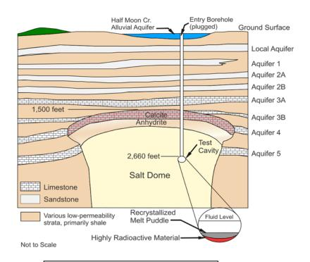
Figure 14. Test Cavity and Aquifers at the Salmon Test Site
